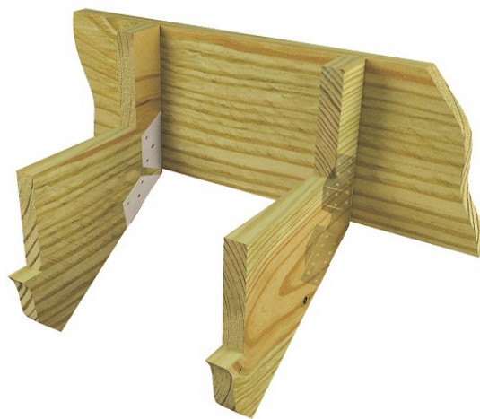
Typical CSH-TZ Installation
